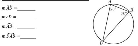
$\angle B$  is the inscribed angle to  $\widehat{AD}$ , so the measure of  $\widehat{AD}$  must be twice the measure of  $\angle B$ .
