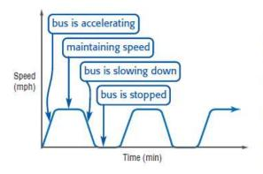
At the origin, the bus is stopped. It accelerates and maintains a constant speed. Then it begins to slow down, eventually stopping. After being stopped for a short time, the bus accelerates again. The process repeats continually.
